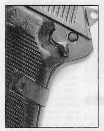
Frame-mounted, three-position safety lever permits the hammer to be safely dropped with a loaded chamber. Horizontally ribbed plastic grip panels are held in place by an odd spring clip.
